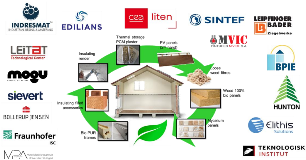
Fig. 1. components to resolve energy loss in a building and the participants in EASI ZERO project.
